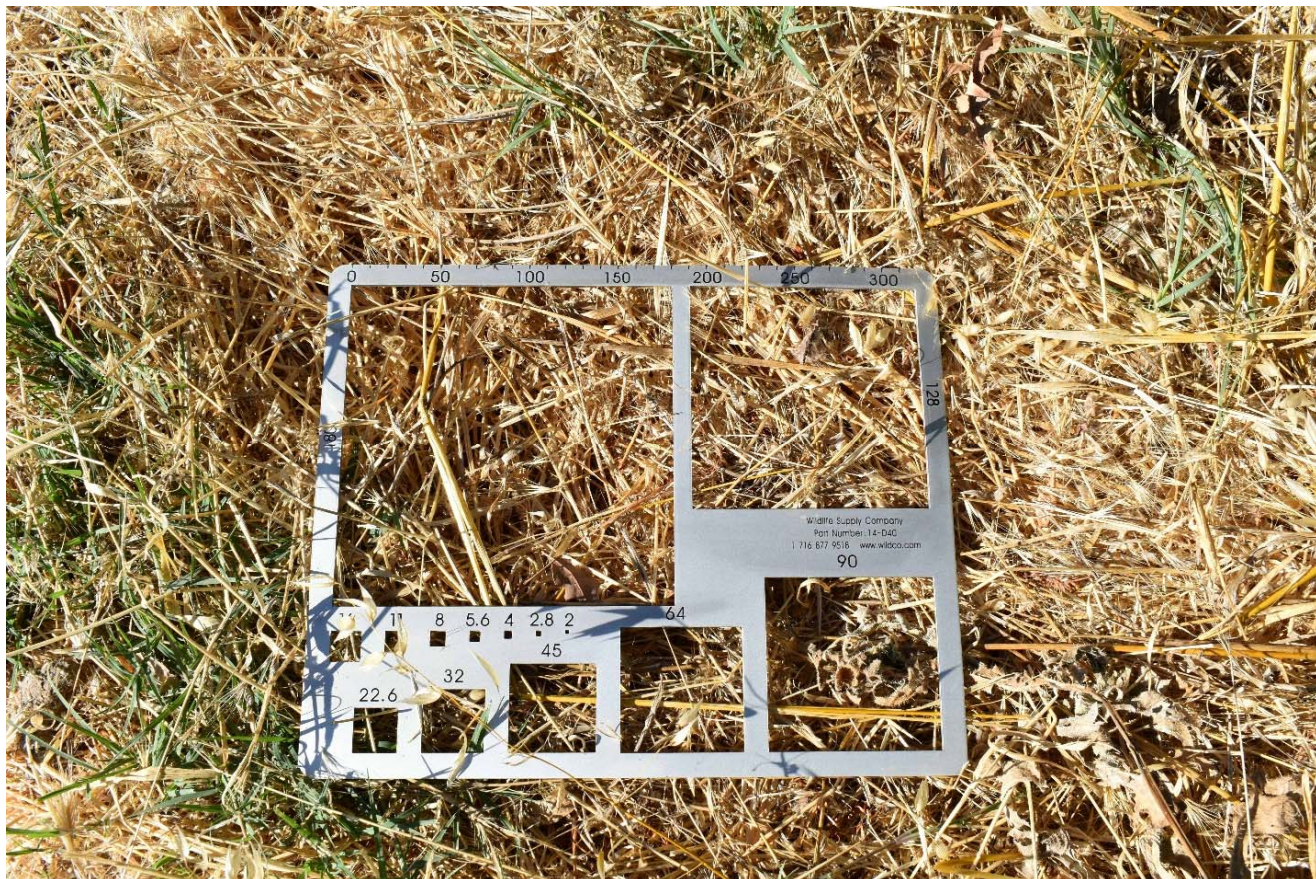
Figure 7. Gravelometer on Channel Bed
