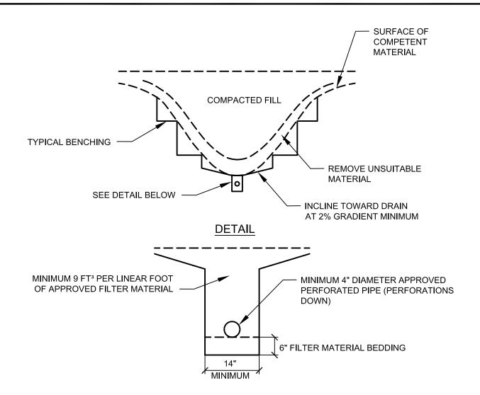
CALTRANS CLASS 2 PERMEABLE MATERIAL FILTER MATERIAL TO MEET FOLLOWING SPECIFICATION OR APPROVED EQUAL:
