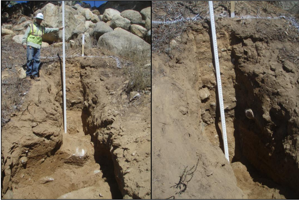
Test Pit TP-5 exposed gravelly/cobbly clayey sand fill, overlying topsoil/colluvium. The test pit met refusal on weathered granitic boulders.
