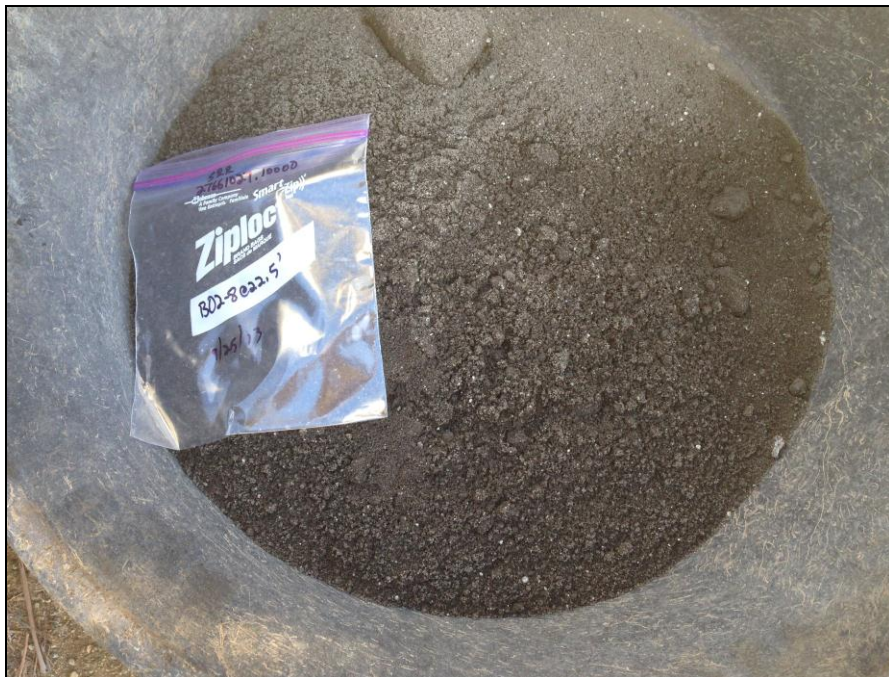
Boring B-2: Sample 8 collected from the Becker cyclone at 22.5 feet. Sample was clayey sand ("dg" soil) collected at the bottom of the embankment fill.
