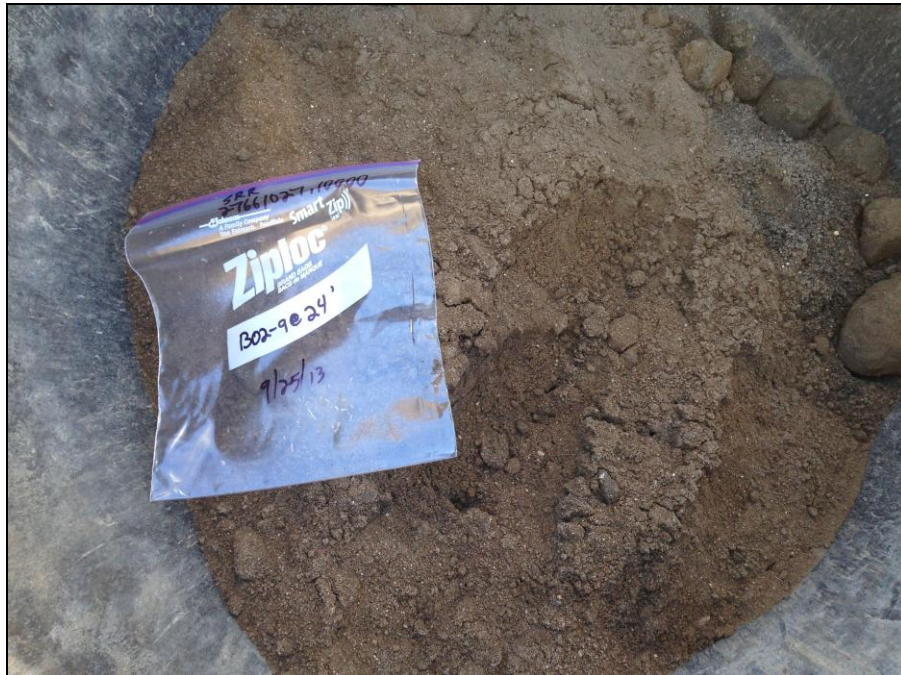
Boring B-2: Sample 9 collected from the Becker cyclone at 24 feet. Sample was collected at the top of highly/completely weathered granitic rock, which breaks down to clayey sand with gravel-sized rock fragments. The Becker open bit allowed continuous logging of the cuttings from the cyclone.
