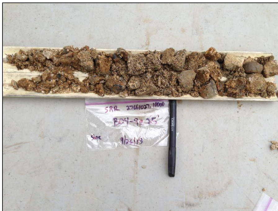
Boring B-4: Sample 9 collected with an SPT sampler at 25 feet. Highly/completely weathered granitic rock about 6 feet below the dam foundation
