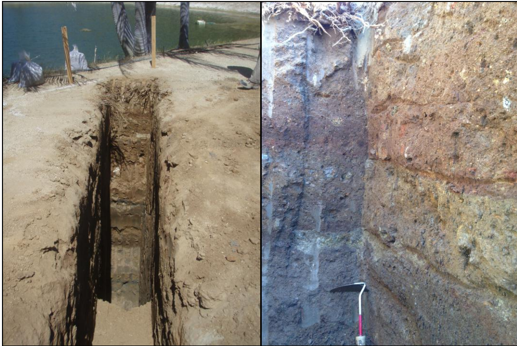
Test Pit TP-2: The embankment fill soil had been placed in thin lifts. The test pit sidewalls appeared stable with no sloughing to the total depth of the excavation (about 14.5 feet bgs),
