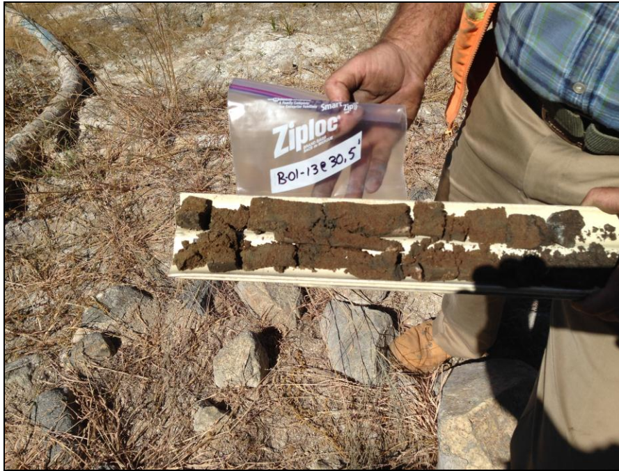
Boring B-1: Sample 13 collected with an SPT sampler at 30.5 feet. Sample was collected at the top of highly/completely weathered granitic rock.
