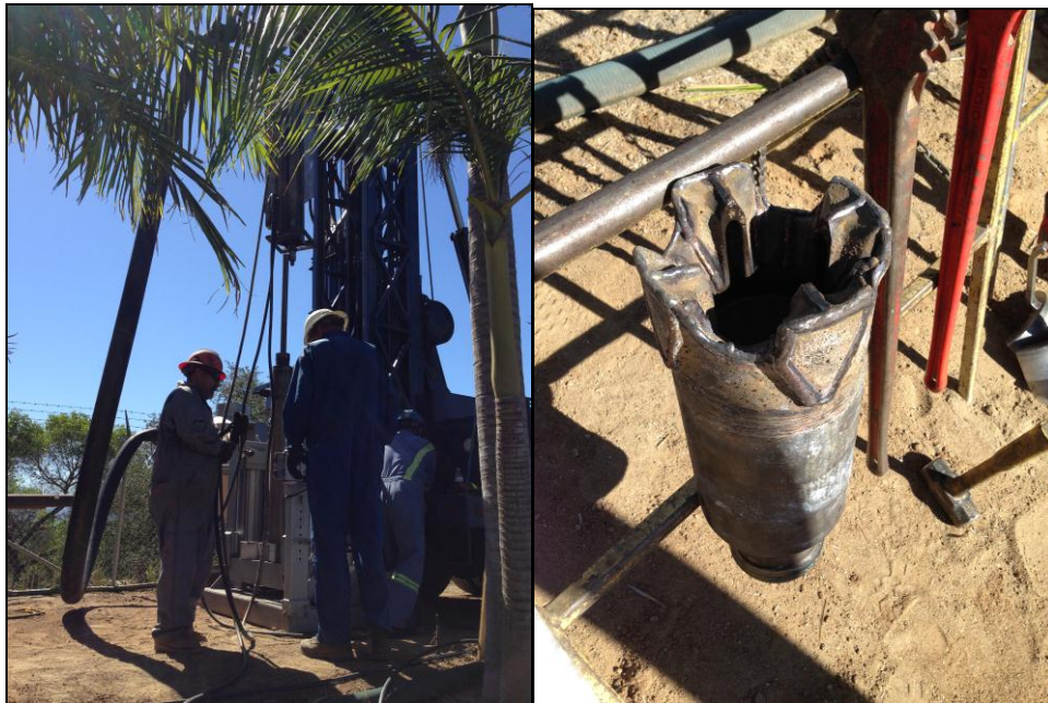
Positioning the 140-lb hammer for SPT sampling (left). The Becker “open bit” on the right.
