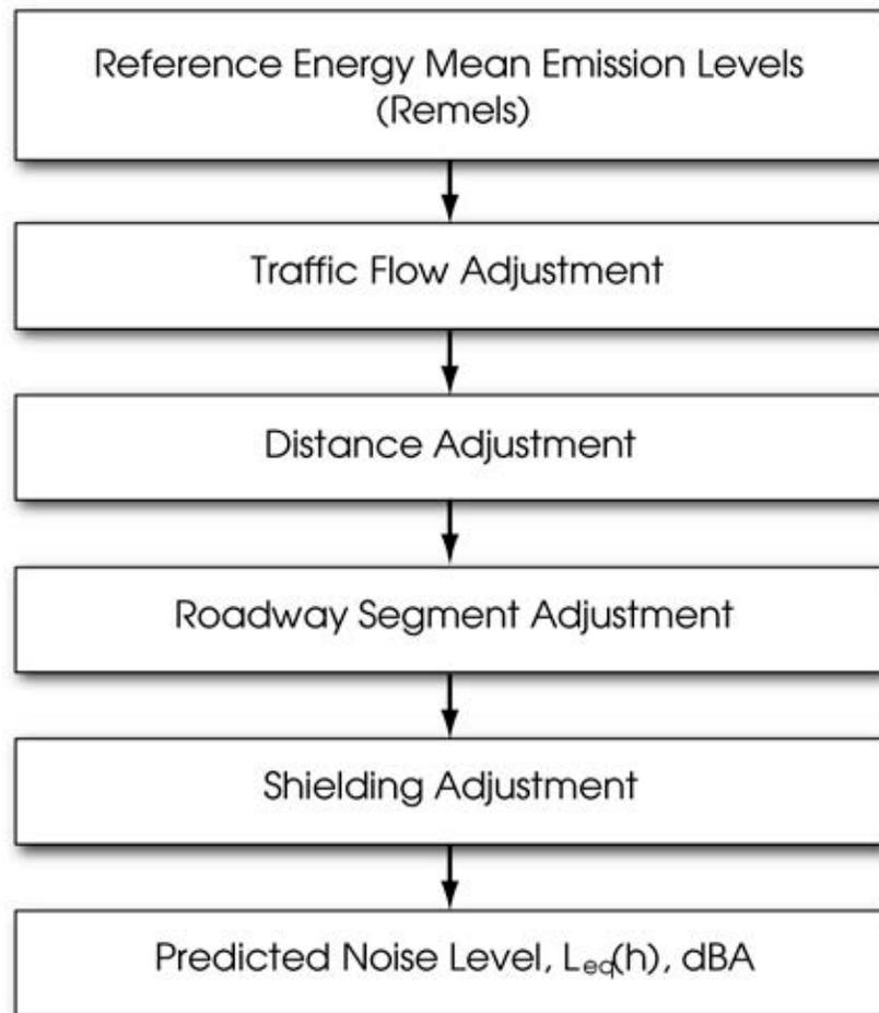
**Figure 5-8.** Flow Chart of FHWA Highway Traffic Noise Prediction Model
