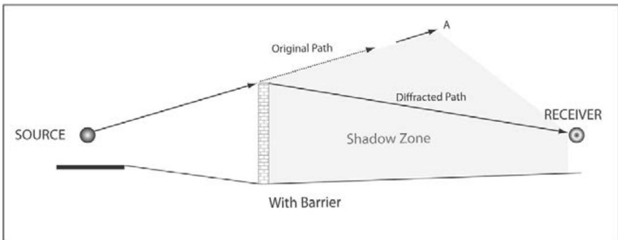
**Figure 6-2.** Barrier Diffraction
