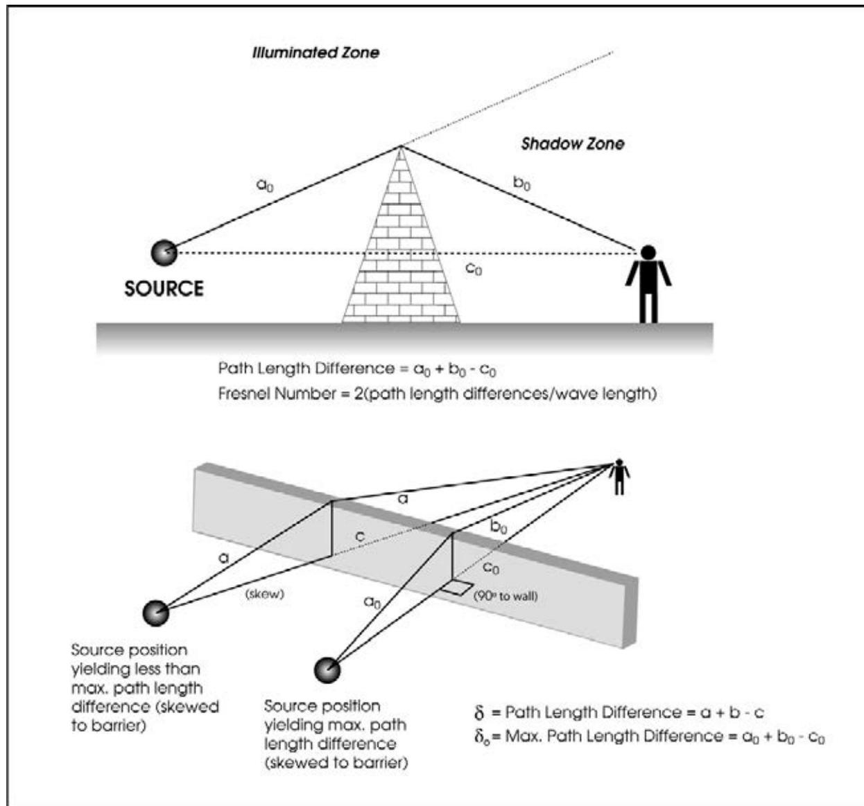
**Figure 5-14.** Path Length Difference and Fresnel Number
