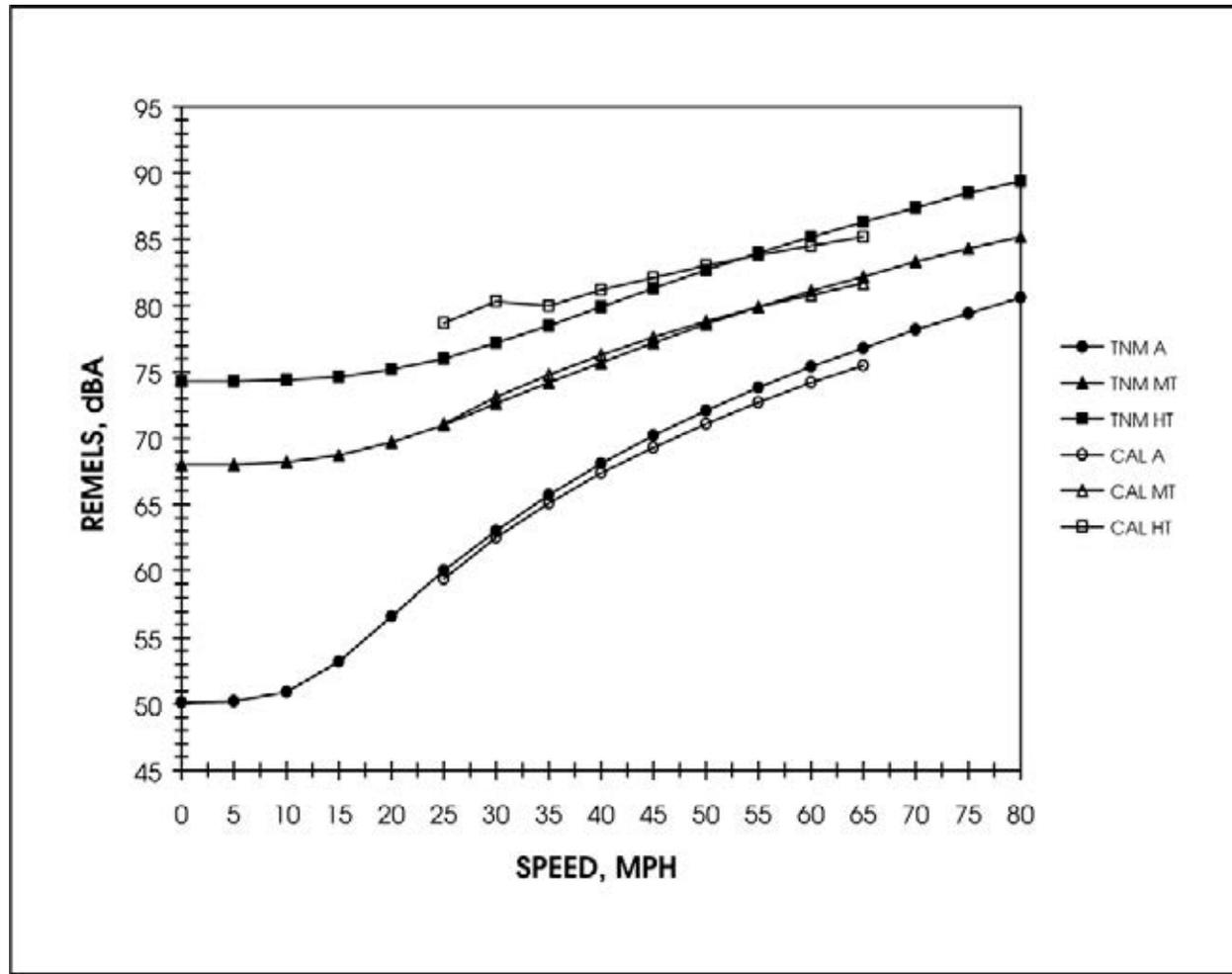
Figure 5-17. Comparison of A-Weighted Baseline FHWA TNM vs. Calven REMELS
