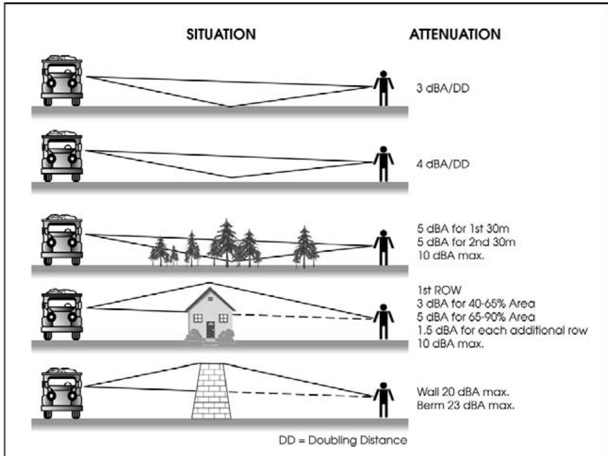
**Figure 5-12.** Shielding Adjustments
