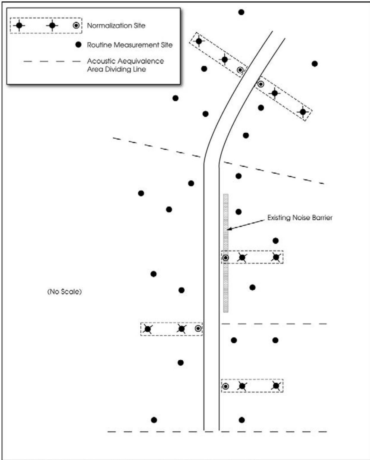
**Figure 5-1.** Normalization Site Selection Map for Three-Microphone Setups
