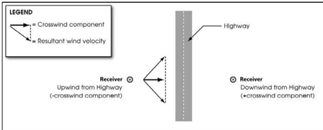
**Figure 5-4.** Plan View of Upwind and Downwind Conditions
