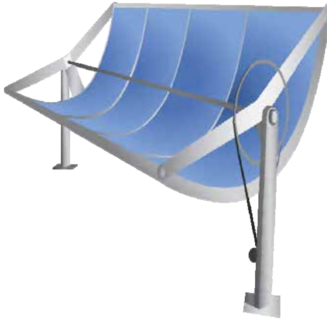
Figure 2: Typical Parabolic Trough Collector
