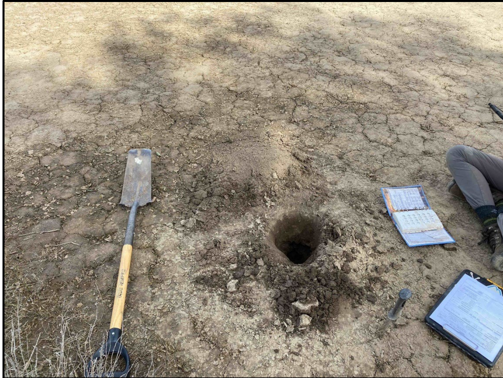
Photograph B57. SP04 examined within isolated unvegetated area. Surface hydrology indicators were observed; however, hydric soils were not present, and the area was determined to lack potentially regulated aquatic resources.
