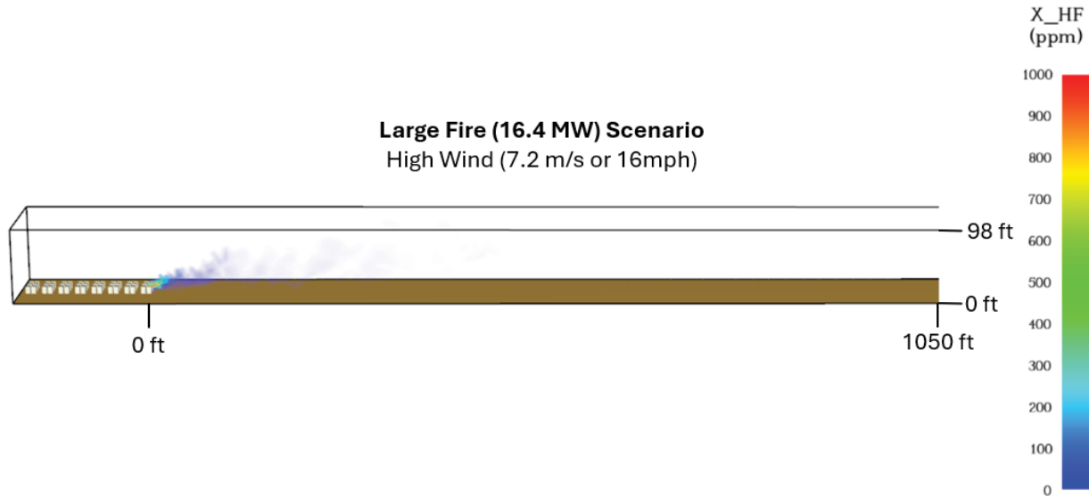
Figure 31: An instantaneous view of the HF in the plume assuming a source term of 43.5 mg/Wh of HF for the large fire high wind, stable scenario. Note that the upper bound of this scale is a factor of 10 lower than in Figure 20.
