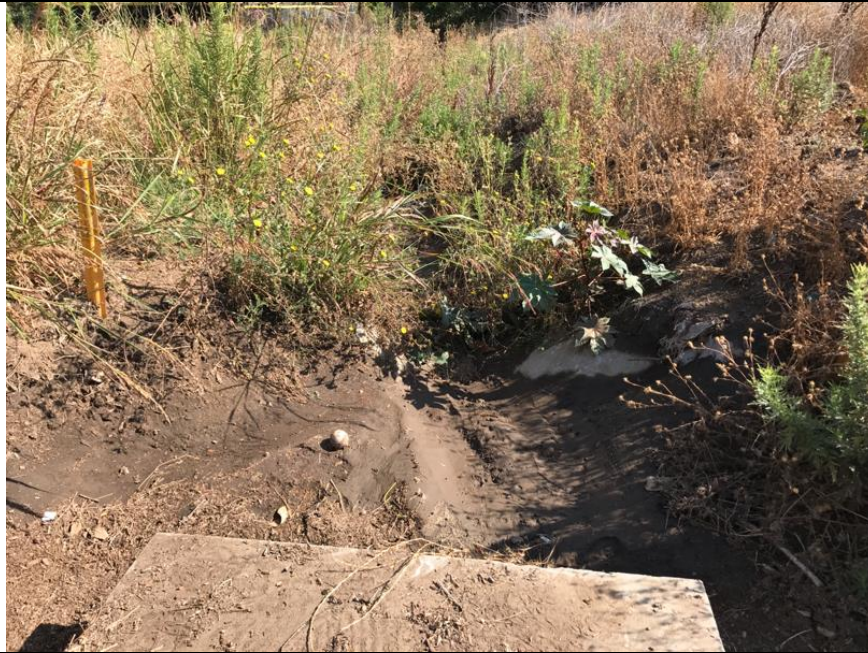
Photograph 1: (33.179, -117.216) North-facing view of the southern reach of the 2-foot-wide earthen-bottom channel on the southern portion of the project site. This photo shows where sampling point NW-1 was taken to determine the presence of OHWM indicators. This photo also shows the approximately 5-foot-diameter concrete culvert that runs south under Hannalei Drive.
