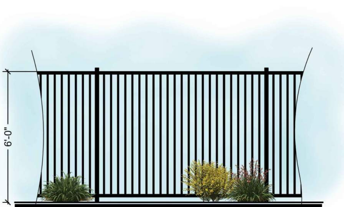
FENCE: W-04 6'-0" TALL TUBULAR STEEL FENCE
