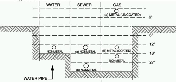
**METAL** – No burial requirement (recommend 12" to protect from mechanical damage and freezing). For copper pipe joints use *only* nonleaded bearing solders (solders approved for potable water).
