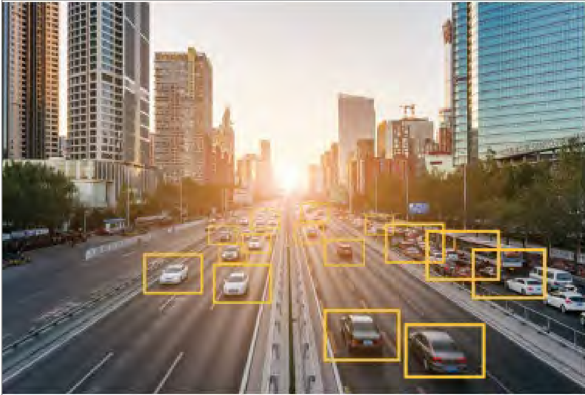
Figure 3 One Rekor camera can capture vehicle reads over multiple lanes of travel.
